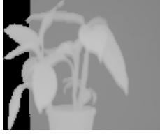
Figure 8. Example of a extracted range image corresponding to the target plant region of the camera image ( 130 \times 113 [pixel]).
