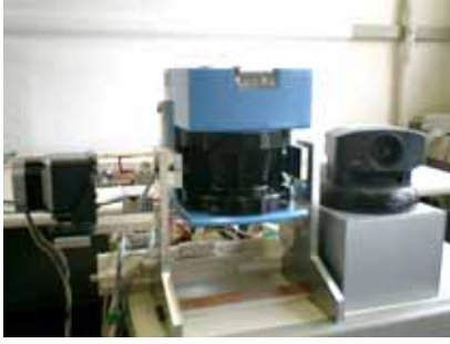
Figure 2. The sensor system consisting of the LRF (center) mounted on the suspension unit, the stepping motor (left), and the PTZ color camera (right).
