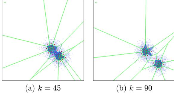
Fig. 4: Voronoi diagrams as results of AVQ of particles. Points and lines represent the weight vectors and Voronoi bounds, respectively.
