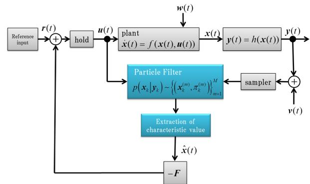
Fig. 1: State variable diagram of the regulator with particle filter.
