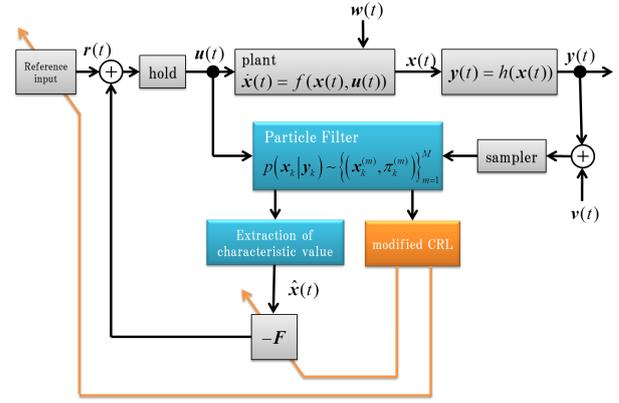
Fig. 2: State variable diagram of the regulator with PF-mCRL.
