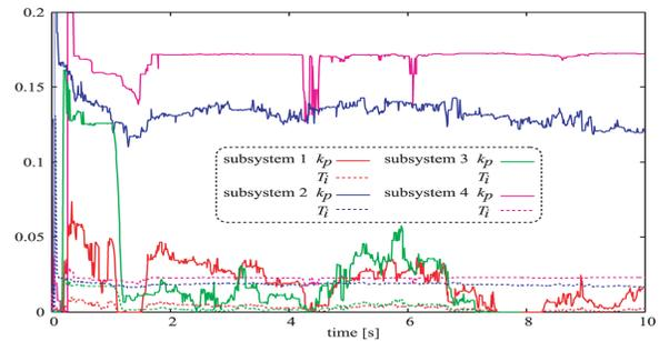
Fig. 6. Time evolution of calculated PI parameters of each subsystem. [Color figure can be viewed in the online issue, which is available at [wileyonlinelibrary.com](http://wileyonlinelibrary.com).]
