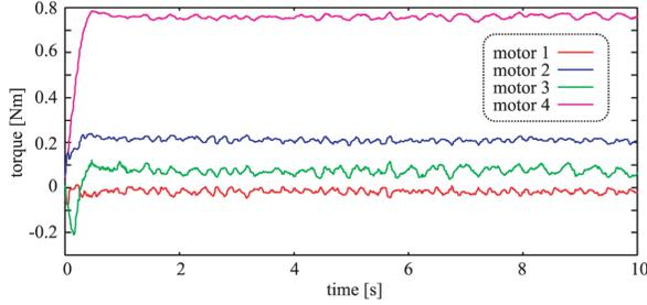
(b) Time evolution of input torques of each motor
