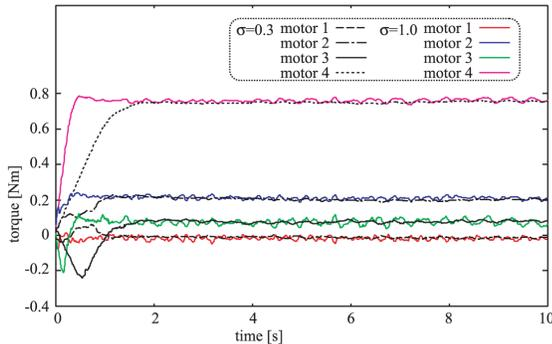
(b) Time evolution of input torques of each motor
