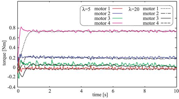
(b) Time evolution of input torques of each motor
