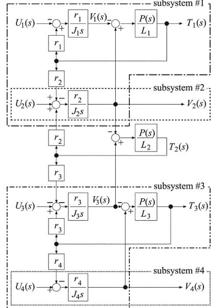
Fig. 2. Block diagram of system.
