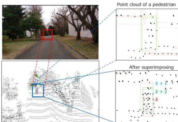
Fig. 9 Superimposing result for pedestrian detection.
