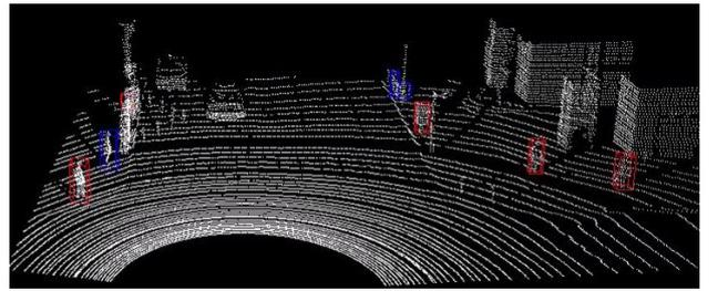
Fig. 5. Example of pedestrian recognition by LIDAR measurement.
