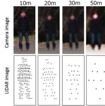
Fig. 4. Example of LIDAR measurement of a pedestrian.
