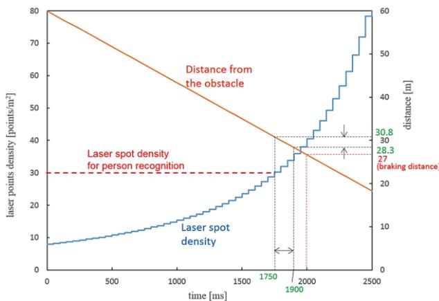
Fig. 3. Relationship of laser spot density and distance.
