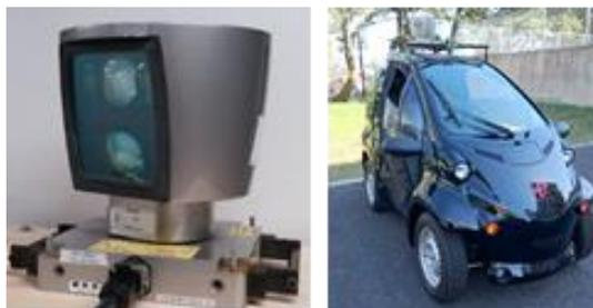
Fig. 2. Overview of Velodyne HDL-64E and a vehicle equipped with the LIDAR.
