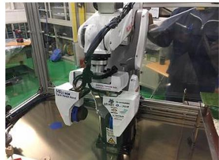
Figure 6. Overview of parallel gripper equipped with cover.
