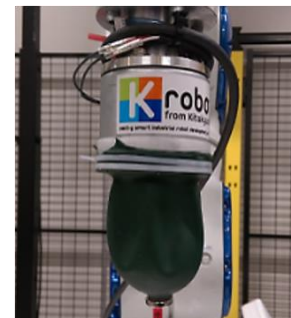
Fig. 4. Overview of water gripper
